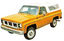
Available in sturdy, weather-proofed canvas with pivoting steel framing for easy stowage, the dealer installed accessory soft top will let you in on the outside world or close up fast when it's cloudy.
