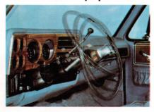
Six-position tilt steering wheel is available with Turbo-Hydra-matic transmissions. Custom 16-inch diameter steering wheel is available in conjunction with power steering.
