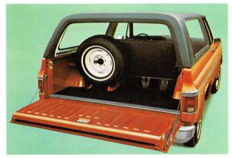
The Jimmy is as wide as a standard pickup and the effective load length behind the drivers seat is 76.6 inches. With the roof off there's room for extra bulky objects, and the load length can be extended by dropping the tailgate which is supported by strap-type steel links.
